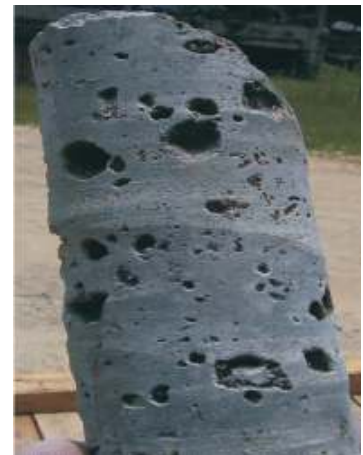
Figure 7 : Photo is showing vugs of different sizes in a hand held slab of the Mfamosing Limestone.
