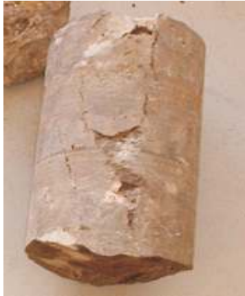
Figure 6: Photo is showing joints and fractures in the Mfamosing Limestone.
