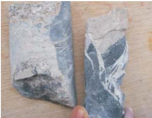
Figure 5: Photo is showing breccia and internal sediments in the Mfamosing Limestone.
