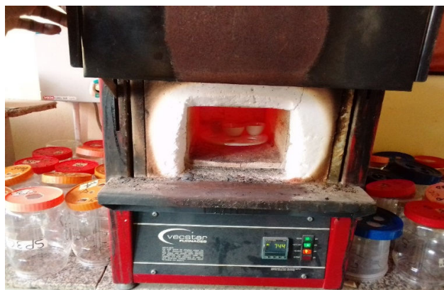
Fig 5: Specimens inside Heat Treatment Furnace
