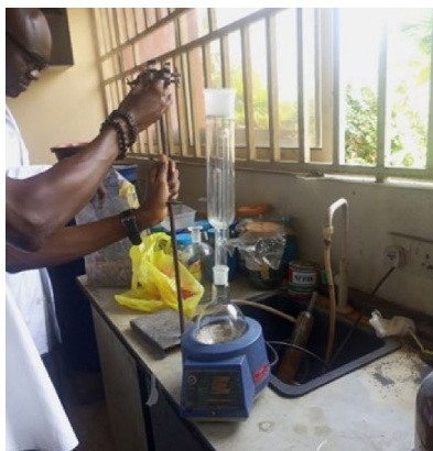
Figure 3: Setting up Soxhlet extraction apparatus
