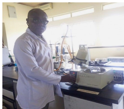
Figure 5: Rotary evaporator for oil separation
